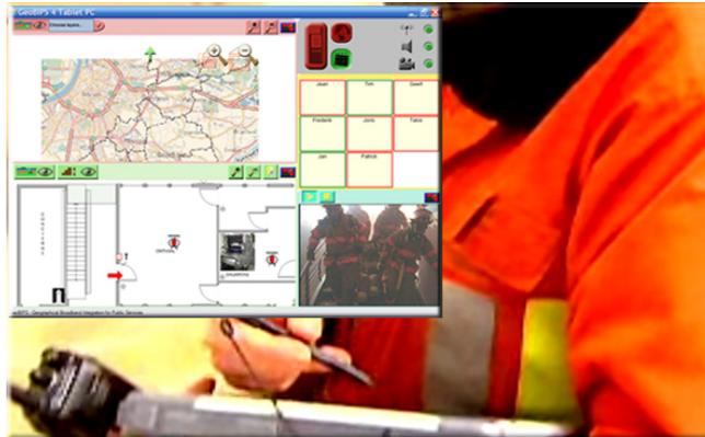
**Fig. 2.** The ruggedized tablet computer is used by the commanding officer and gives an overview of the situation including the status of the different team members of the fire brigade at the intervention site
