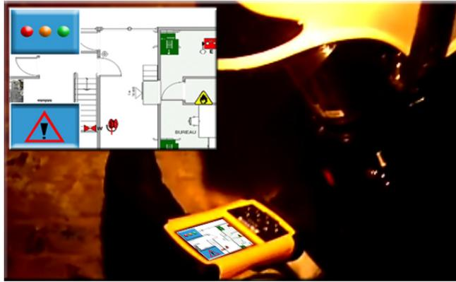
**Fig. 1.** The ruggedized PDA shows the floorplan and shows the status of the explosion
