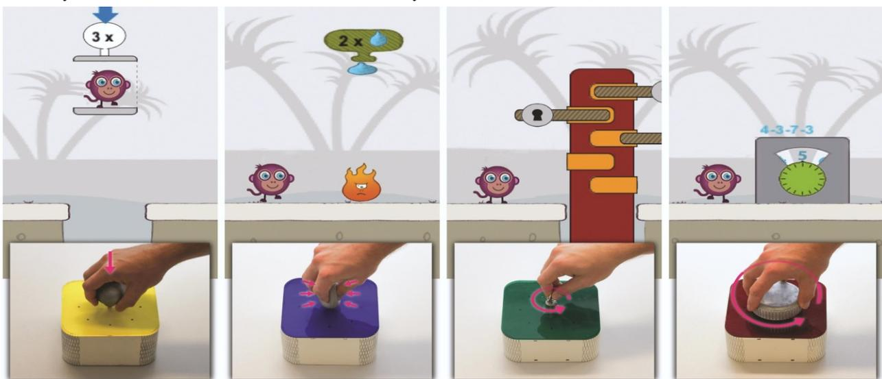
Figure 5. With Handly, we designed game elements to provide strong visual cues and natural mappings that integrate four different hand tasks as its core interaction techniques. This makes the interface easy to understand and use.
