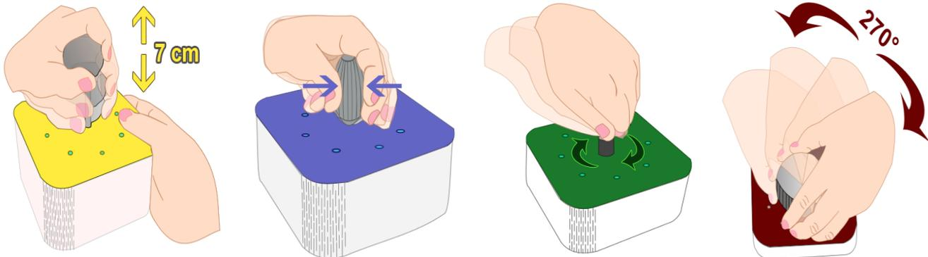
**Figure 3. Overview of movements and ranges of motion with (A) push and pull, (B) squeeze, (C) key turn and (D) knob turn.**
