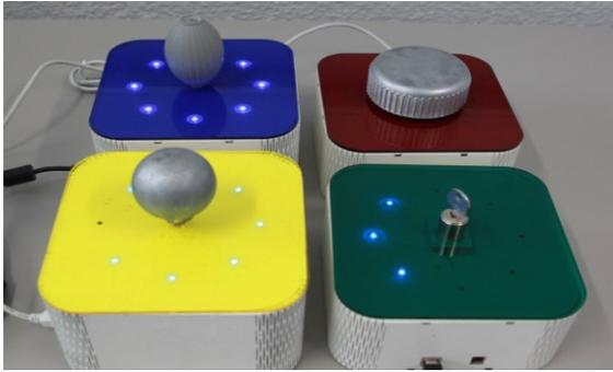
**Figure 2. Four tangible training boxes with embedded sensors and feedback for different handgrips and tasks.**
