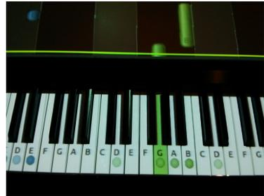
Figure 2: Keys that need to be played are highlighted with a colored circle. The circle's opacity gradually increases as the scrolling note gets closer. When the scrolling note reaches the key, the entire key is highlighted.
